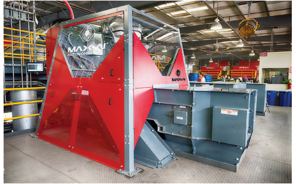
MAX, one of two AI robots at Athens' Material Recovery Facility in Sun Valley, sorts recyclable material from trash in order to reduce what winds up in a landfill.
