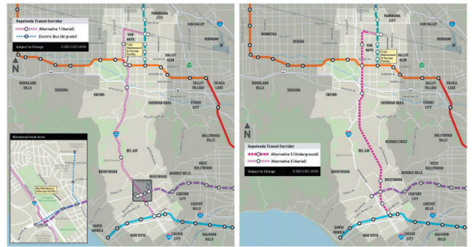
Two alternatives for the Sepulveda Transit Corridor Project, one proposing an above ground monorail (left) and another proposing underground heavy rail with a dedicated UCLA station (right). Photos courtesy of Metro
